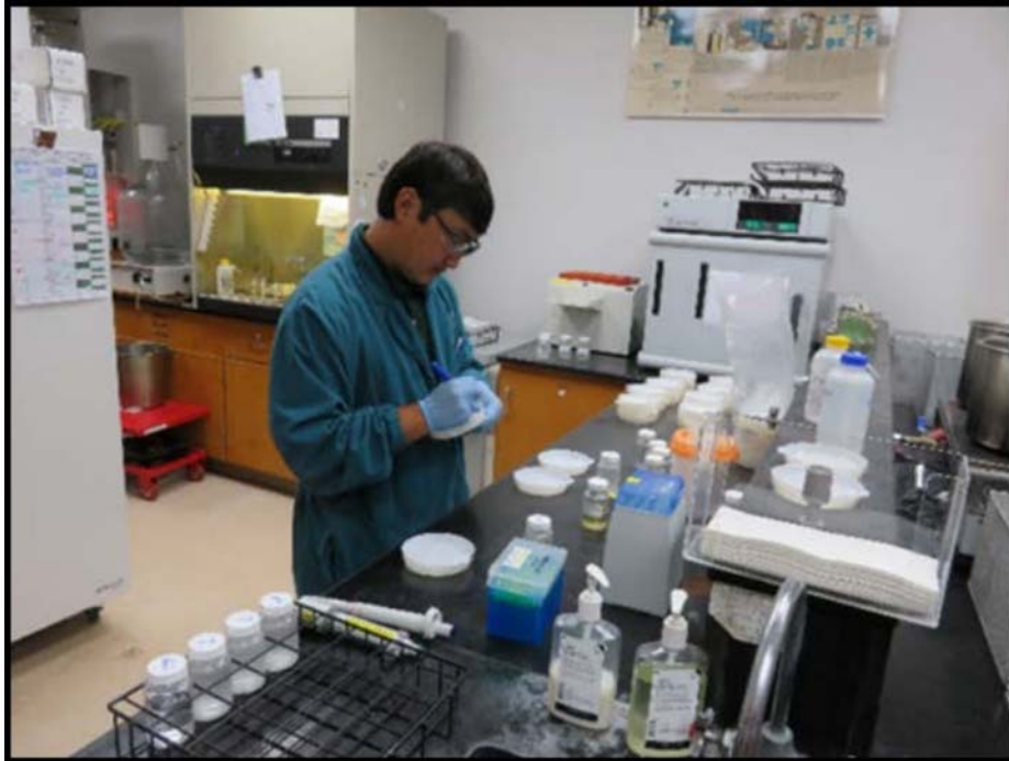
Christopher Kawaguchi, Water Microbiologist I, setting up Sim-Plate HPC (heterotrophic plate count) for routine bacti- analysis
